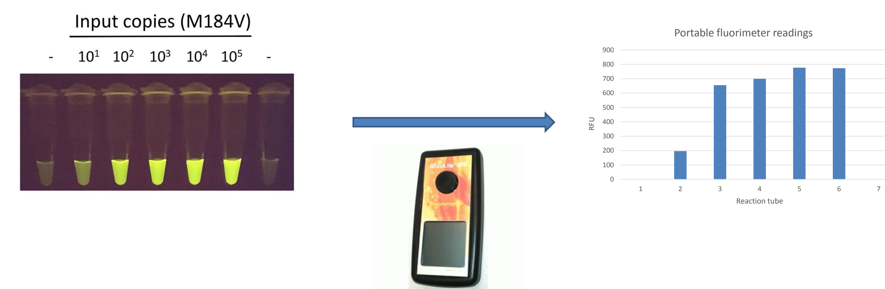
Figure 4. Enhanced AS-PCR for HIV-1 resistance mutations is highly sensitive. Representative results using M184V template dilutions demonstrating detection of low copy number target. Fluorescence intensity can be quantified using a portable, battery-powered fluorimeter.
